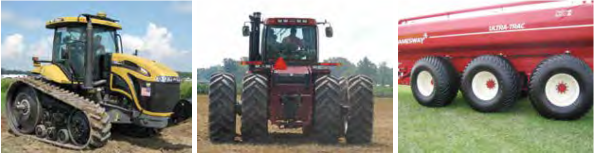
Figure 15.7. Reduction of soil compaction by increased distribution of equipment loads. Left: Tracks on a tractor. Middle: Dual wheels on a tractor that also increase traction. Right: Multiple axles and flotation tires on a liquid manure spreader.
