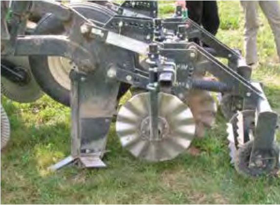
Figure 16.9. Left: A strip-till tool with hilling disks and rolling basket to create a zone of loosened soil. Photo by Robert Schindelbeck. Right: Strip-till after corn harvest results in a narrow tilled zone that leaves much of the soil surface undisturbed. Photo by Georgi Mitev.
