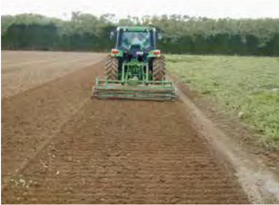
Figure 16.6. Powered tillage tools used with horticultural crops: Left: rotary tiller; Right: A spader.
